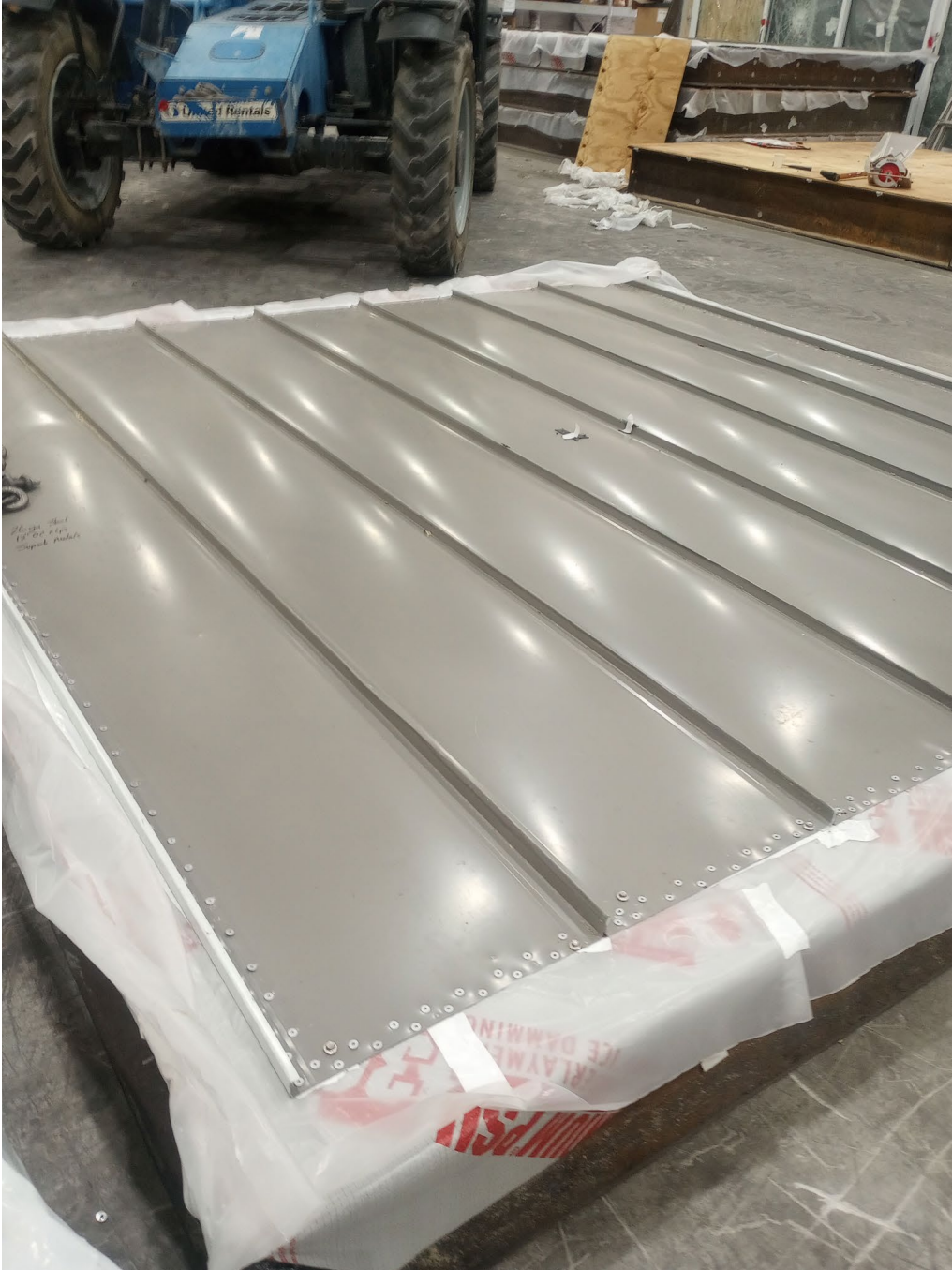
Photo No. 1 26GA Test Deck After Testing
